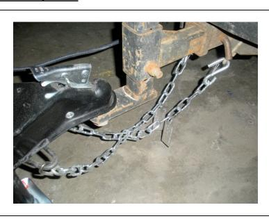
Visually inspect the safety chains and hooks for wear or damage. Replace worn or damaged safety chains and hooks before towing.
